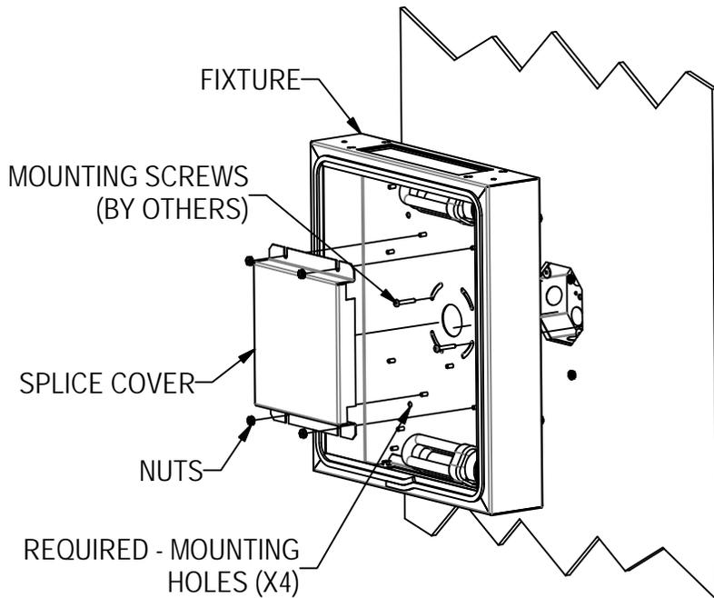
1. REMOVE (4) FOUR NUTS AND SPLICE COVER TO MOUNT FIXTURE TO J-BOX, WITH HARDWARE (BY OTHERS).
